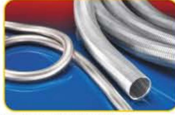
METAL HOSE INOX 376 <math><10^3 \Omega</math> 600° C ID : 20 mm...300 mm
