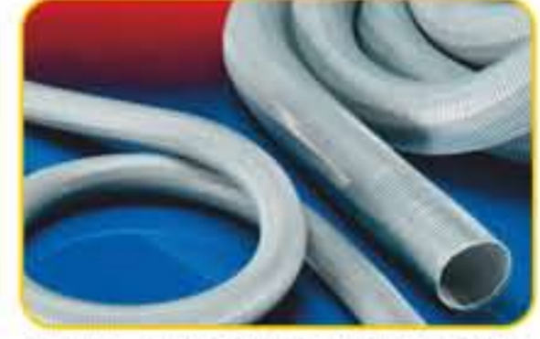
METAL HOSE 377 REINFORCED <math><10^3 \Omega</math> 600° C ID : 50 mm...300 mm
